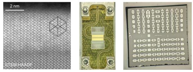
From left to right: Cross-sectional transmission electron microscope view of a 6 nm thick epitaxial film of Bi-doped iron garnet [Collab. U. Zaragoza]; Device for cryogenic microwave magnetization dynamic experiments on extended films; Nano-fabricated chip with several types of magnonic devices.
