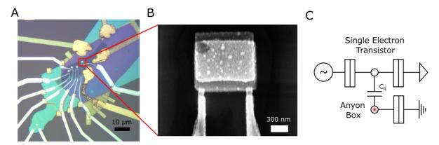
**A.** Optical image showing multiple single electron detectors (white) capacitively coupled to bilayer graphene equipped with electrostatic gates made of 2D materials. **B.** Scanning electron microscope image of an aluminum single electron transistor realized at the Néel Institute. **C.** Schematic of the measurement showing the anyon box capacitively coupled to the single electron transistor.
