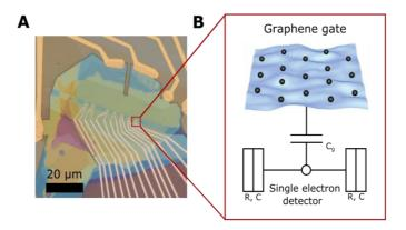
**A.** Optical image showing multiple single electron detectors (white) capacitively coupled to bilayer graphene equipped with electrostatic gates made of 2D materials. **B.** Schematic of the measurement showing a lattice of anyons (black dots on blue background) capacitively coupled to a single electron transistor.
