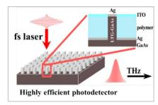
**Research topic:** The aim of the proposed M2 internship is to participate in the design, the fabrication and the test of an original optoelectronic component (see reference and figure) dedicated to the excitation of flying qubit using ultra-short single-electron charge pulses. The work will be done in close collaboration in between Institut Néel (fabrication of the device, time resolved quantum experiment) and IMEP-LAHC (design and test of the THz photodetector).
