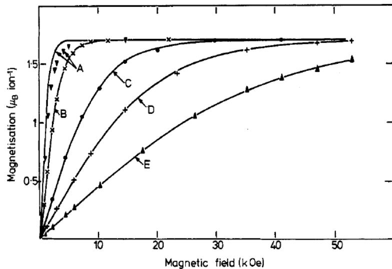
Figure 3. Magnetisation against applied field at various temperatures for YbGaG;  $H \parallel [111]$ . The experimental values are indicated by different types of points. A, 0.17 K; B, 0.38 K; C, 1.16 K; D, 2.17 K; E, 4.2 K. The full curves represent the calculations performed with an isolated ground-state doublet.
