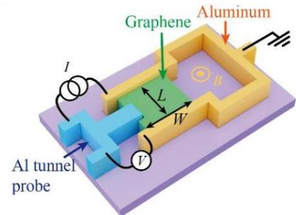
**Figure 1.** Schematic of an Al-based tunneling probe used to study graphene-based Josephson junction. Figure taken from [4].
