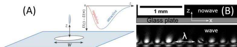
(A) Typical configuration of Casimir repulsive: an object facing a micro-hole. The associated force-distance curve is shown. (extract from [1]). (B) Evanescent acoustic field in the
