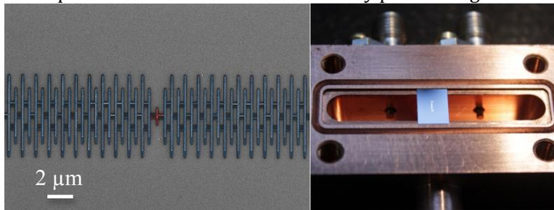
*Left: example of a Josephson meta-material we engineer in our lab [1]. It is made of thousands of Josephson junctions and behaves as a “superinductance”, which is several orders of magnitude larger than what is usually found in standard electronic circuits. Right: superconducting qubit embedding a superinductance (black rectangle) sitting in its copper microwave cavity. In this specific case, the addition of a superinductance enabled a novel readout mechanism.*
