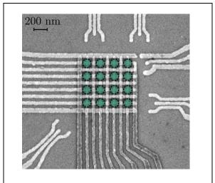
2D array of Quantum dots using 2 layers of gates on GaAs
