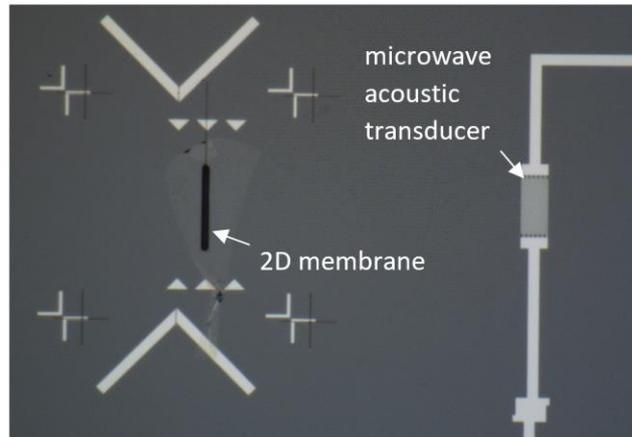
*Left: room temperature characterization of acoustic devices at GHz frequencies, performed before cooling the devices down to mK temperatures. Right: An acoustic device recently developed in the lab. A transducer made out of superconducting circuits (white color) is used to launch and detect acoustic waves, in order to acoustically probe a suspended 2D membrane.*
