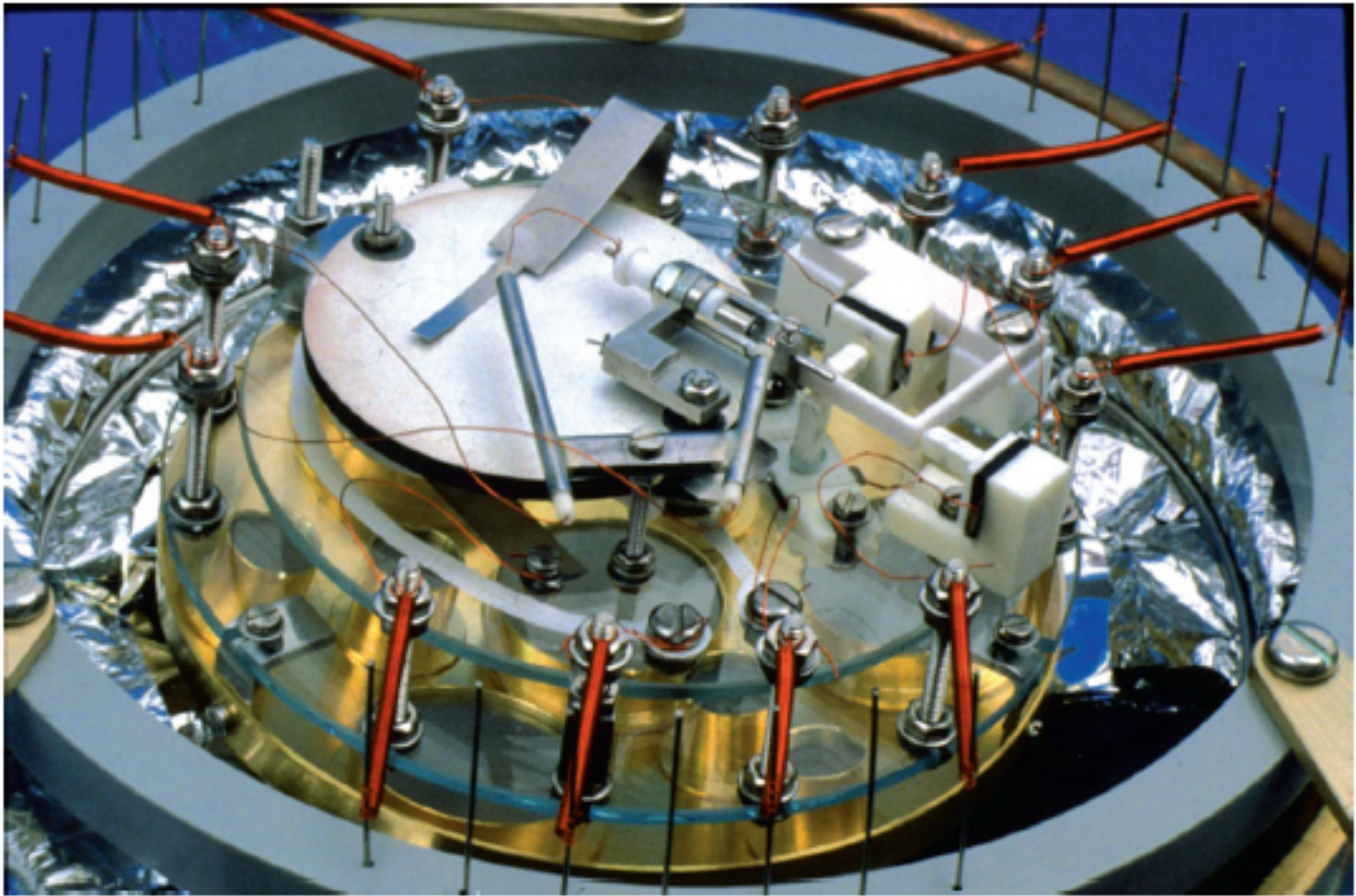
Fig. 2: Close-up of the first scanning tunneling microscope built in 1981. (courtesy of IBM Zurich Research Laboratory)
