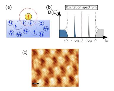
Figure 1: (a) Illustration of the competition of superconducting pairing with the magnetic exchange coupling provided by an isolated impurity. (b) Density of states at the impurity site, displaying the resulting Yu-Shiba-Rusinov bound states, at energies helow the superconducting gap. (c) STM image ofgraphene superconducting rhenium, which on top of the atomic structure. a moiré superstructure is seen. This demonstrates the high structural coherence of graphene rhenium.
