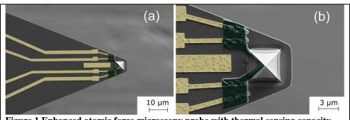
Figure 1 Enhanced atomic force microscopy probe with thermal sensing capacity.
