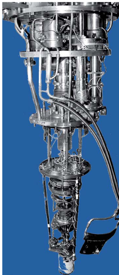
Fig. 1 : This autonomous dilution refrigerator, free from cryogenic fluids, has a base temperature of less than one-hundredth of a degree above absolute zero.
