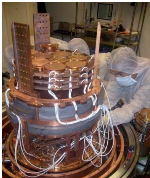
Fig. 1: In the Modane underground Laboratory (LSM), the Edelweiss II experiment has successfully accomplished the first cooldown of its cryostat and recorded the first background pulses from its detectors. This experiment is dedicated to the search for the Dark Matter of our galaxies.
