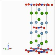
Figure 1: Unit cell of Ca<sub>2</sub>CuO<sub>2</sub>Cl<sub>2</sub> (Cu blue, O red, Cl green, Ca cyan), with the square unit of the CuO<sub>2</sub> plane visible, where the superconductivity take place.
