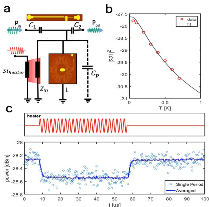
Figure 1: (a) Electric diagram of the RF thermometry scheme, involving a superconducting LC resonator in parallel with the temperature-dependent impedance  $Z_{Si}$ . A neighboring Si cell is used as a heater. (b) Temperature dependence of the resonator transmission and fit using the independently determined  $Z_{Si}(T)$ . (c) Real-time response of resonator transmission to a heating pulse, demonstrating  $\mu$ -scale thermometry.
