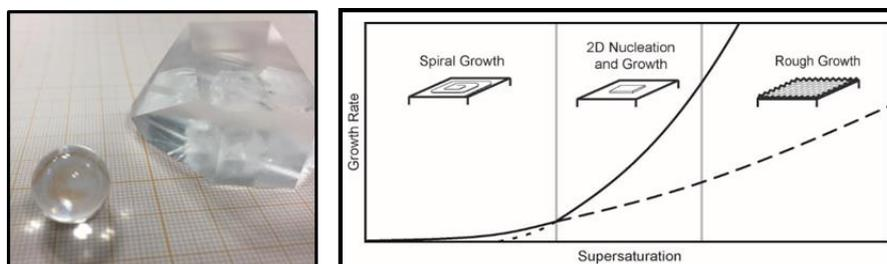
Figure 1: a)  $\text{KH}_2\text{PO}_4$  bulk crystal and sphere shaped sample obtained from that crystal and b) growth mechanism as a function of supersaturation.
