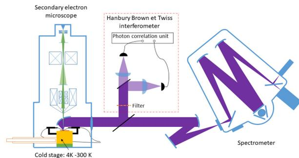
Figure 1 -Schematic diagram of the CL setup as well as the photon correlation module
