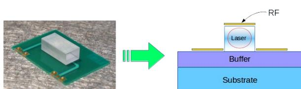
*Bulk oxides doped with rare-earth ions can be advantageously replaced by semiconductor doped matrices to shrink the device to micro-size scale and then benefiting from a strong optical and RF field confinements for qubit addressing.*
