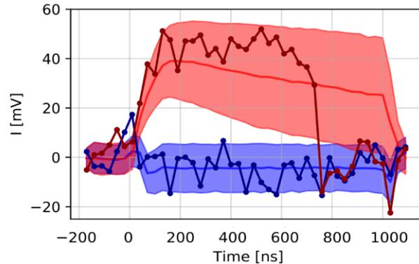
Figure: Quantum trajectories (successive single shot measurement) when the qubit is prepared in its ground state  $|g\rangle$  (blue points) and excited state  $|e\rangle$  (red points) at  $t=0\text{ns}$ . A quantum jump is observed at about 750ns.
