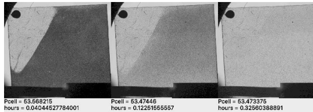
Optical signature of the stochastic nature of hexane cavitation in nanoporous alumina membranes
