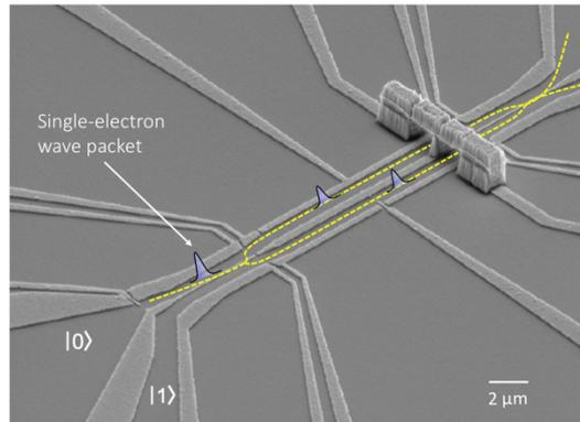
Fig. 1. Scanning electron micrograph of a Mach-Zehnder type quantum interferometer operating as a flying qubit. A single-electron wave packet is prepared in a given quantum state (here  $|0\rangle$ ) and injected in one of the arms of the interferometer and put into a quantum superposition.
