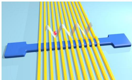
*Figure: Artistic view of the sample envisioned to realize a multi-dot structure to perform operations and algorithms with a few electron spin qubits.*
