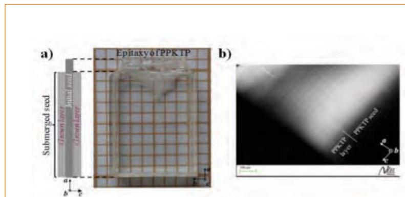
Figure 2 : Periodically domain-structured-KTP films grown on a PPKTP seed in a  $0.1 \text{KTP} - 0.6 \text{KPO}_3 - 0.3 \text{KF}$  flux. a) Photograph of a PPKTP crystal and, at left, a cross-section showing the growth seed and its crystallographic axes. b) Scanning Electron Microscope image of the PPKTP seed and the grown layer.
