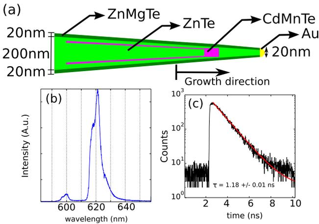
**Figure 1.** (a) Nanowire morphology: an Au droplet serves as a catalyst to grow a CdTe quantum dot inserted in a ZnTe conical nanowire. A lateral regrowth of ZnMgTe creates a shell around this core. (b) Typical  $\mu$ PL spectrum of a nanowire QD and (c) corresponding decay rate measurement, integrating a bandwidth of 10 nm around 622 nm. A monoexponential fit (red line) gives a lifetime  $\tau = 1.18 \pm 0.01$  ns.
