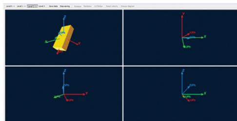
Fig. 1. The upper left corner shows an image of level 1 (see text) while the three other parts show projections of unit vectors attached to the smartphone ( $x_{iPh}$ ,  $y_{iPh}$ ,  $z_{iPh}$ ) in OXY, OZY, and OXZ planes defined in the lab frame.
