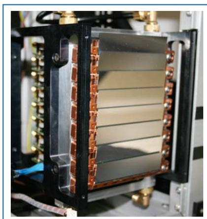
Figure 1 : Inside a prototype Silicon XPAD3 detector : 8 modules are tiled as close as possible to each other to offer a 7x12 cm<sup>2</sup> detection surface with almost 540000 pixels of size 0.13x0.13 mm<sup>2</sup>.
