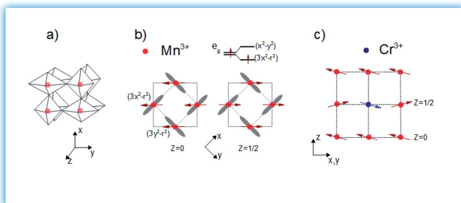
Fig. 1: (a) The 3D structural scheme of alternate, Jahn-Teller distorted  $\text{MnO}_6$  cages in the orthorhombic crystal  $\text{LaMnO}_3$ . (b) Ordering of the  $e_g$  orbitals (represented in grey) and magnetic orderings (red arrows) in the  $ab$  plane for  $z=0$  and  $z=c/2$  (where  $z$  is the crystal  $c$ -axis). (c) Our proposed solution for the ferromagnetic ordering observed when an Mn is replaced by a Cr impurity.
