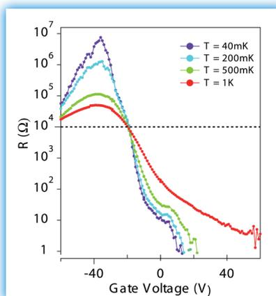
Fig. 2: Effect of varying the perpendicular electric field for various temperatures showing 7 orders of magnitude of resistance tuning at the lowest temperature. The large dynamic contribution of the conductance within the graphene layer enables us to observe a temperature-dependent transition from superconductor (at positive gate voltage  $V$ ) to insulator at negative  $V$ .
