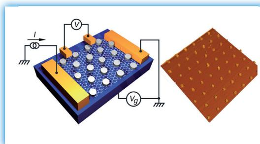
Fig. 1. **At left** : Principle of a graphene transistor with tin disks (not to scale) decorating a graphene plane; the electrical properties are measured with four gold electrodes. **At right**: Atomic Force Microscope (AFM) micrograph of the central, active part of the device showing the triangular array of Sn dots.
