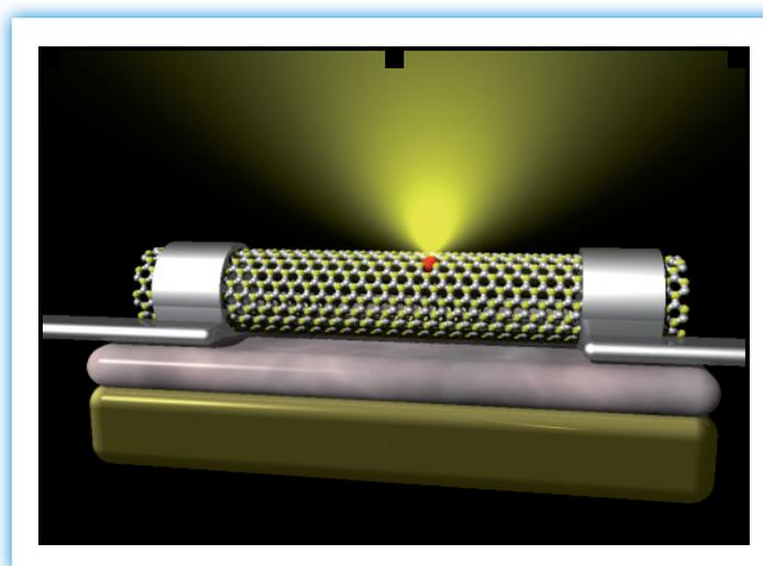
Fig. 2: Schematic set-up for the proposed method of activating an optoelectronic device based on Boron Nitride nanotubes with lattice defects (red dot). The method uses an ambipolar transistor configuration. BN nanotubes are deposited on an insulating surface that acts as a gate dielectric to enable application of the transverse electric field that controls the wavelength of the light emission.
