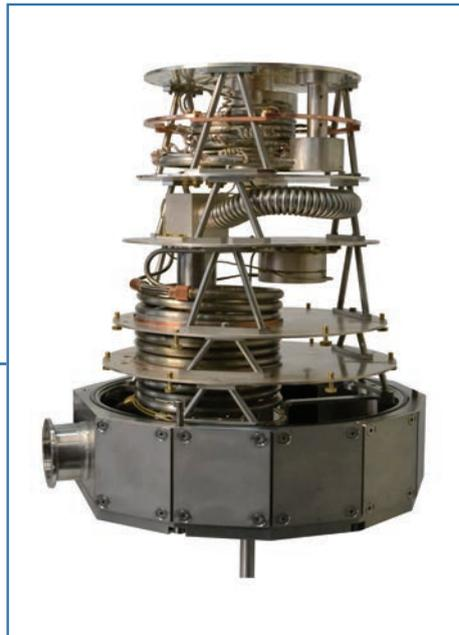
New generation of the Sionludi table-top dilution cryostat, with its thermal shields and outer vacuum container removed. The compact, inverted design allows the cryostat to be mounted on a bench top. The sample space is located on top of the upper plate, making it easily accessible.
