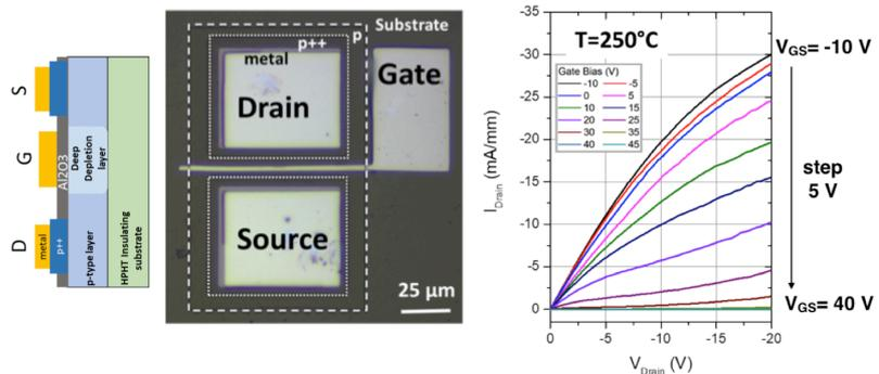
From left to right: Schematic cross section, top view optical image and characteristics of a deep depletion diamond MOSFET.
