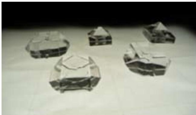
Crystals of Deuterated KDP of size several  $\text{cm}^3$  obtained by rapid growth in solution under stationary conditions.
