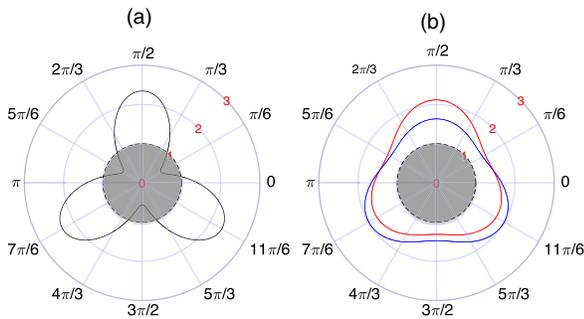
FIG. 2. Gain (a) and  $\hat{P}_k$  (red) and  $\hat{Q}_k$  (blue) variances (b) as a function of the phase of the seeding fields, for  $|\xi| = 1.75 \times 10^{-6}$  and  $\bar{N}_{\text{in}} = 4 \times 10^{10}$ . The gray circles indicate the unity gain in (a) and the standard quantum limit in (b).
