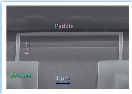
Fig. 1: Scanning Electron Microscope (SEM) image of a silicon NEMs sample of "goalpost" type. The 7 μm long "paddle" bar is 150 nm thick x 250 nm wide, and 30 nm of aluminum is evaporated on the top surface. It vibrates out-of-plane thanks to the electromagnetic excitation force (magnetomotive scheme).
