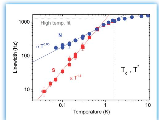
Fig. 2: An aluminium coated Si cantilever structure reaches quality factors  $f/\Delta f$  of order one million around 20 mK, exceptional for a mechanical mode resonating around 10 MHz. N and S denote measurements with the Al in normal and superconducting states, while  $T^*$  (which happens to coincide with  $T_c$ , aluminium's critical temperature) marks the beginning of the damping decrease as  $T$  is reduced.
