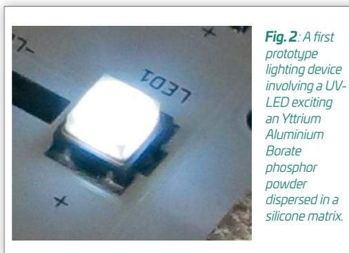
**Fig. 2:** A first prototype lighting device involving a UV-LED exciting an Yttrium Aluminium Borate phosphor powder dispersed in a silicone matrix.
