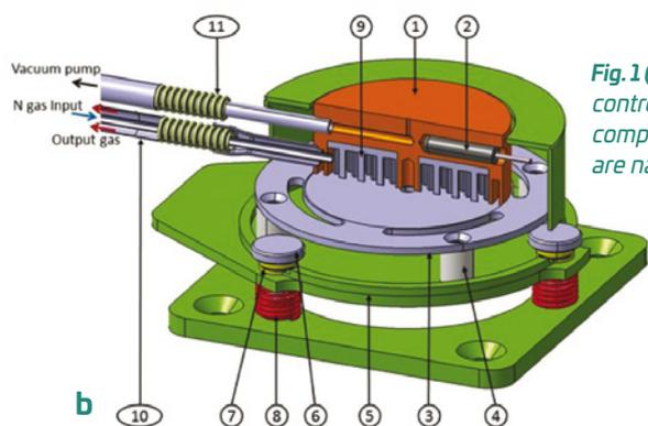
**Fig. 1 (b):** The temperature-controlled sample-holder component. Items A-F and 1-11 are named in the text.
