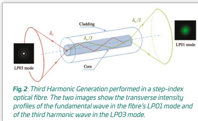
**Fig. 2:** Third Harmonic Generation performed in a step-index optical fibre. The two images show the transverse intensity profiles of the fundamental wave in the fibre's LP01 mode and of the third harmonic wave in the LP03 mode.
