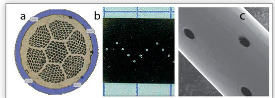
**Fig. 2:** (a) Cross-section of a 0.8 mm diameter multi-filament Bi-2212 wire with our 50  $\mu\text{m}$  thickness reinforcing sheath in Inconel (blue). (b) Inconel strip material with zigzag pattern of holes. (c) Tube-like sheath formed by rolling the Inconel strip round the wire and stretching it to fit; the holes (elongated by the stretching) enable oxidising heat treatment of the wire.
