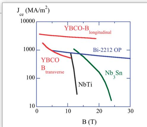
Advances in High Temperature Superconductors are changing the situation. These ceramic materials, with values of  $T_c$  up to around 100 K, can outperform metallic superconductors when used at liquid Helium temperature. In particular, "YBCO" (Yttrium Barium Copper Oxide) and "Bismuth-2212" (Bismuth Strontium Calcium Copper Oxide,  $\text{Bi}_2\text{Sr}_2\text{CaCu}_2\text{O}_x$ ) can remain superconducting up to very high current densities at 4 K, even under very high fields  $B$ , see Fig. 1.
