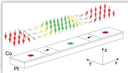
In this scenario, the second ingredient needed for efficient wall motion is a phenomenon called the Spin Hall effect that produces a spin-polarized electron current flowing from the Pt to the Co layer when an electrical current passes through the Pt layer. This spin current flow generates a strong torque that moves all the chiral walls in the same direction through the cobalt layer.
