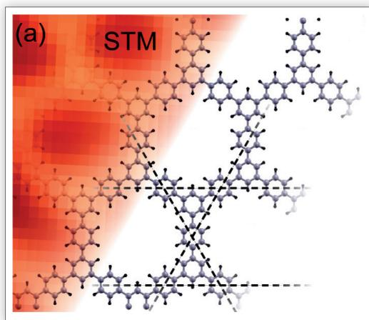
**Fig. 1:** At top left, a Scanning Tunnelling Microscope image of a nanoporous network grown on a gold substrate. The superimposed schema at bottom-right shows the interpretation of this image: a hexagonal symmetry 2-Dimensional network of chains of benzene rings enclosing large “pores”.
