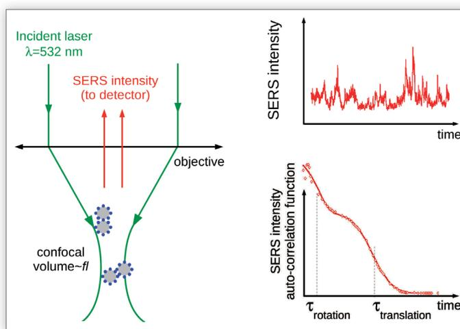
**Fig. 1:** At left: A microscope illuminates a colloidal solution of nanoparticles (grey circles) carrying adsorbed molecules (blue dots). The Surface Enhanced Raman Scattering by the molecules, in the backwards direction, is recorded as a function of time (top right). The auto-correlation function (bottom right) yields rotational and translational characteristic times related to the geometry of the diffusing objects.
