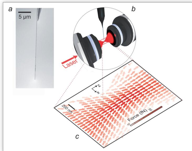
**Fig. 1:** (a) Scanning Electron Microscope image of a 150 nm diameter Silicon Carbide nanowire, suspended at its top on a tungsten tip.
