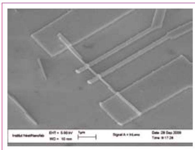
Connected thermoelectric nanowires.
