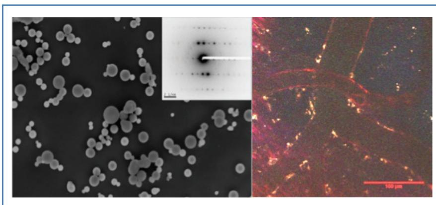
Figure 2 : (a) Scanning Electron Microscope image of nanoparticles prepared from a sprayed sol-gel solution containing CMONS organic dye. Insert in (a): typical electron diffraction pattern showing that the organic cores are single crystals of CMONS. (b) First in vivo, two-photon fluorescence angiography of the microvasculature of the brain of a mouse.
