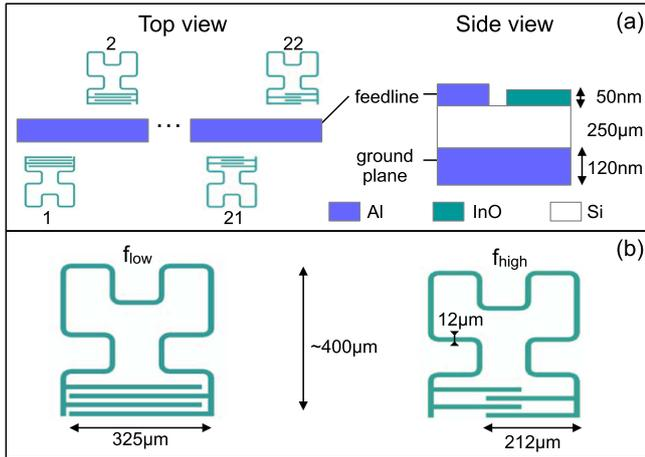
**Figure 1.** Resonators' design. (a) Twenty-two devices are coupled to the common feed-line. Cross-section view of the micro-strip configuration. (b) Detailed design of the  $f_{\text{low}}$  and the  $f_{\text{high}}$  resonators. The Hilbert fractal inductor is identical for all the resonators. The four capacitor fingers length are varied from one resonator to another: from the shortest ( $f_{\text{high}}$ ) to the longest ( $f_{\text{low}}$ ).
