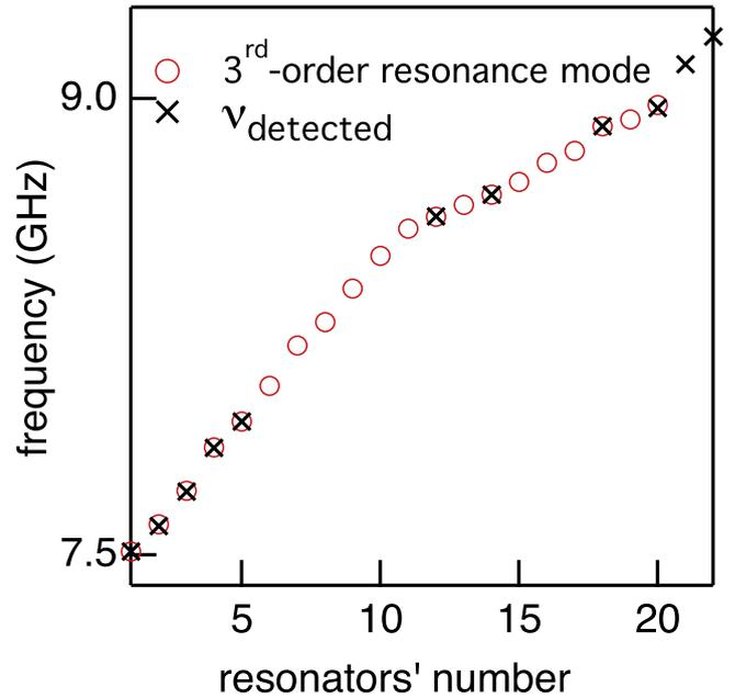
**Figure 3.** GHz sub-gap detection tunability. As a function of the resonator number the  $\nu_{detected}$ -frequency compared to third-order resonance mode identified with a  $f_{VNA}$ -scan. From one resonator to the next the total length varies by  $\sim 10 \mu\text{m}$ . The  $f_{VNA}$ -scan was measured up to 9 GHz. The  $\nu_{detected}$ -frequency was probed for 11 resonators.
