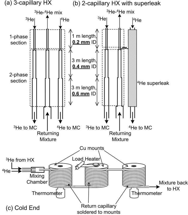
Figure 2: (a), (b) The two counterflow heat-exchanger designs tested. (c) The cold end of the fridge (not to scale), used with both heat exchangers. (MC: Mixing chamber, HX: Heat exchanger.) The thermometer on the left measures the mixing chamber temperature; the thermometer on the right measures the temperature of the mixture after absorbing the heat load,  $T_{load}$ .
