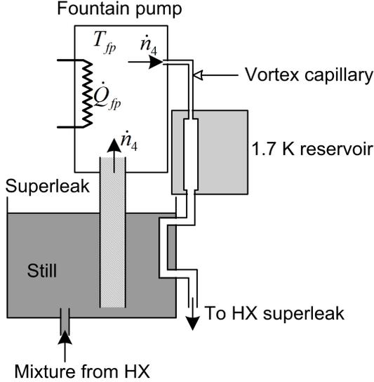
Figure 5: The fountain pump and the  $^4\text{He}$  circulation loop. Superfluid  $^4\text{He}$  flows through the superleak from the still into the fountain pump, drawn by the fountain effect. A heat input  $\dot{Q}_{fp}$  is applied to the fountain pump. Bulk  $^4\text{He}$  flows out of the fountain pump and is cooled, first in the 1.7 K reservoir and then in the still, before making its way down the heat exchanger.
