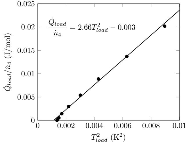
(b)  $\dot{Q}_{load}/\dot{n}_4$  vs  $T_{load}^2$
