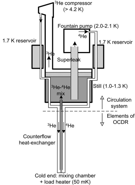
Figure 1: A schematic of the closed-cycle gravity-independent dilution refrigerator.
