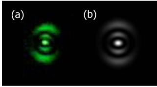
Fig. 2. Measured (a) and calculated (b) transverse distributions of the third-harmonic  $LP_{03}$  mode propagating in the 183-mm-long fiber at 516 nm.
