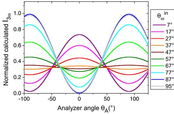
Fig. 7. Normalized calculated third-harmonic energy generated in the 642-mm-long fiber plotted as a function of the analyzer angle  $\theta_A$  for different values  $\theta_\omega^{\text{in}}$  of the input linearly polarized fundamental wave.
