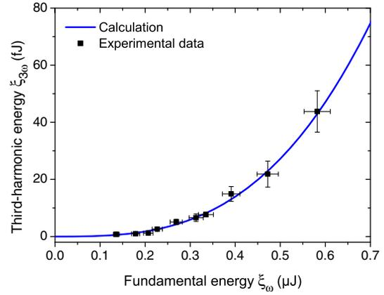
Fig. 4. Third-harmonic energy generated in the 642-mm-long fiber as a function of the fundamental energy.
