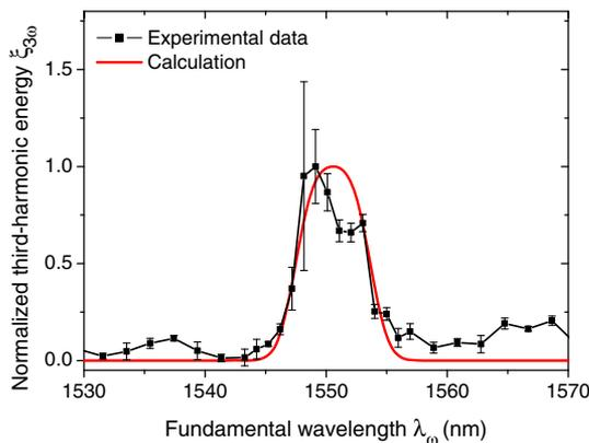
Fig. 3. Third-harmonic energy generated in the 183-mm-long fiber as a function of the fundamental energy around phase matching.
