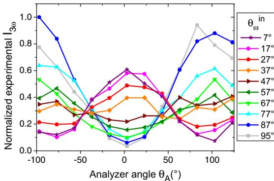
Fig. 6. Normalized measured third-harmonic energy generated in the 642-mm-long fiber plotted as a function of the analyzer angle  $\theta_A$  for different values  $\theta_{\omega}^{\text{in}}$  of the input linearly polarized fundamental wave. The error bars of the measurements are not put for more clarity; the corresponding uncertainty is of about  $\pm 5.5\%$ .
