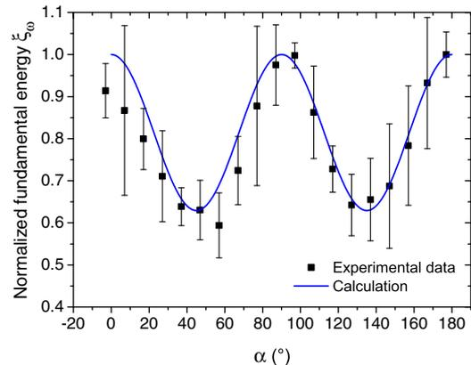
Fig. 5. Fundamental energy  $\xi_\omega$  transmitted by the 642-mm-long fiber placed between parallel polarizer (half-wave plate) and analyzer (Glan–Taylor prism).  $\alpha$  is the corresponding rotation angle of polarization.
