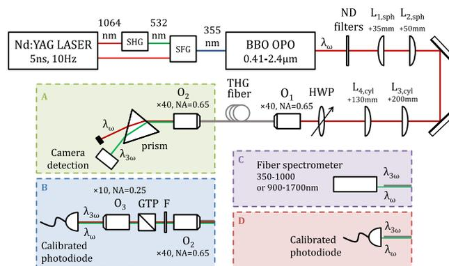
Fig. 1. Experimental setup used for the THG study: ND stands for neutral density, L for lens, HWP for half-wave plate,  $O_i$  for microscope objective, F for dichroic filters and GTP for Glan-Taylor polarizer; the different units are used for specific measurements: A for the modes imaging, B for the polarization configuration, C for the spectral properties, and D for the conversion efficiency.
