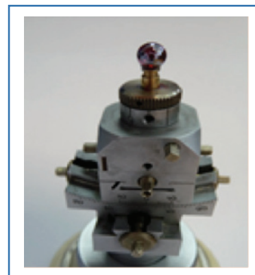
Figure 2 The 5-mm-diameter \text{CdSiP}_2 sphere placed on the top of a high precision angular positioning stage.
